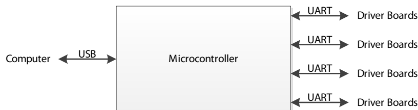
Figure 3.33.: The communication channels on the controller board.
